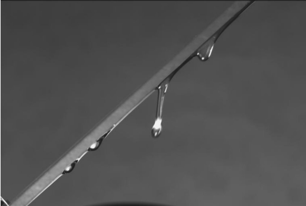
FIGURE 3. Fall-off at \theta_c by the pinch-off mechanism. The last hump is barely supercritical while the first two are barely subcritical. The subcritical drops traverse the entire plane without falling off. Different drops are on different sides of criticality because, at this critical condition, a fallen drop can reduce the local flow rate to subcritical values. ( \theta = 42^\circ , v = 2.18 \text{ cm}^2 \text{ s}^{-1} , q = 2.27 \text{ cm}^3 \text{ s}^{-1} .) The critical \theta_c is 45^\circ for these conditions.
